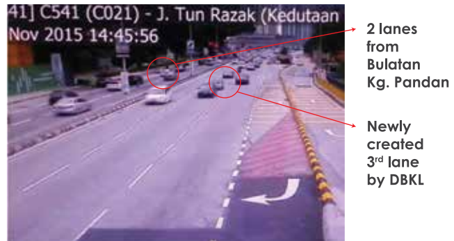
Figure 10: Jalan Tun Razak in front of US Embassy, Physical barrier to overcome weaving problem in front of the US Embassy
