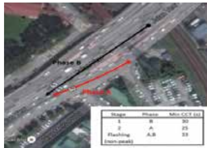
Figure 16: Installation of Ramp Metering System (RMS) at ramp up from Jalan Yew roundabout.
